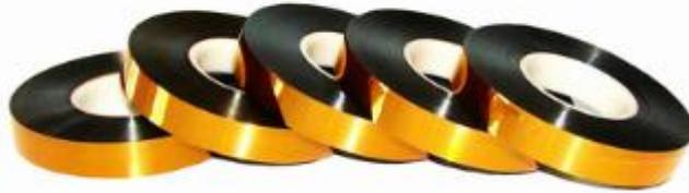
Polyimide pressure sensitive adhesive tape with silicone resin, This kind of tape is made of polyimide material with heat-resistant silicone adhesive, which shows excellent dielectric insulation properties, high heat resistant, excellent solvent resistant, mask-off gold finger contacts during wave soldering, short-term temp. 250c x 5sec, and is widely used for electrical insulation on motor, transformer, coils, PCB making and so on.
